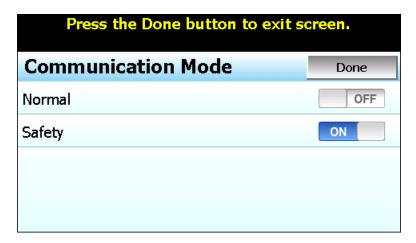
With the **Normal** mode selection, the loop control will continue operation according to the last command given. When power is first applied to the MCT4, the loop control outputs will activate immediately according to the last commands given prior to power loss.
