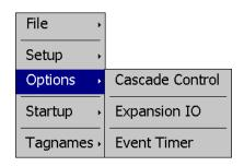
The **Options** menu provides access to Cascade Control, Expansion IO and Event Timer configuration settings.
