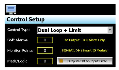
The **Control Type** drop down menu is used to define the mode of operation for the MCT4. The number of PCM process loop boards and HLM limit board (if required) are set automatically and dependent upon the control type selected. The selections include:
