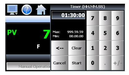
If the run time is one hour and thirty minutes, enter a value of 13000 for 1 hour, 30 minutes and 00 seconds. One hour and thirty minutes can also be interpreted as a total time of 90 minutes; therefore, you can also enter a value of 9000 for 90 minutes, 00 seconds. Upon pressing the 'Start' button, the timer will begin operation and the countdown will be displayed and begin as 1:30:00.
