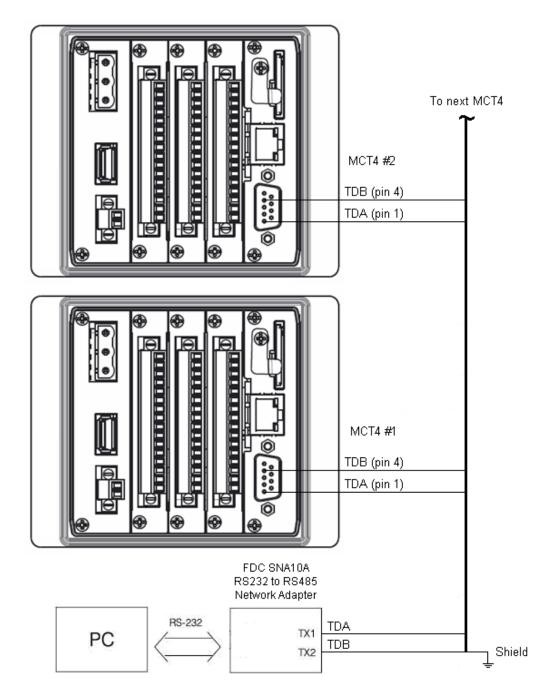
**NOTE:** The connection requires a single twisted-pair cable that is daisy-chained from one MCT4 to the next. When using shielded twisted-pair cable, be sure to ground only one end of the cable, preferably at the RS232 to RS485 network adapter. Allowing any other portion of the cable shield to come in contact with ground, or grounding both ends, will cause ground loop currents to flow in that section of the cable which can cause communication errors.
