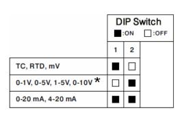
\*0-1V and 0-5V/1-5V input types are special order. HLM units ordered with either input type cannot be programmed for any other type.
