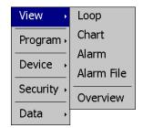
The **View** menu provides navigation to all standard view screens. These include the Loop view, real time Chart, Alarm monitor, Alarm File and Overview control screens.
