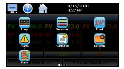
Slide page 1 provides navigation to all standard view screens. These include the Loop and Overview, Chart, Alarm monitor, and Alarm File.
