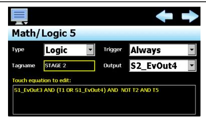
By duplicating the stage 1 equation and appending the requirement that the system 2 delay time has expired (represented as T5), the stage 2 compressor output will activate and deactivate under the same conditions as the stage 1 compressor, but also require the system 2 delay to be expired. Since the system 2 delay timer is only enabled if stage 1 is active and the humidity system is not active, the permits stage 2 operation only when in heat/cool operation and not humidity operation as required.
