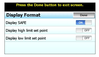
When **Display SAFE** is selected, the Loop View and All View screens in the runtime application will display the word "SAFE" when the limit alarm is not active. When a limit alarm is activated, the word "SAFE" will be replaced with either the high limit set point (if the high limit alarm is tripped) or the low limit set point (if the low limit alarm is tripped).
