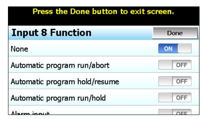
The **Automatic program run/abort** function will start the currently loaded program from step 1 if not already running, upon activation of the input (an off to on transition). Deactivating the input (an on to off transition) will stop the program if it is currently running.
