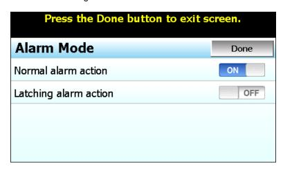
Normal alarm action has the alarm output off in the non-alarm condition and on in the alarm condition.
