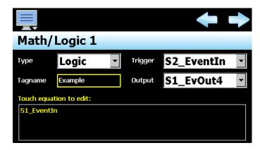
As long as loop 2 event input is true (on), the equation will be evaluated. Thus, the loop 1 event output 4 will be on when the loop 1 event input is on and off when it is off.
