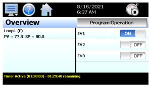
To stop the timer, press the "Stopwatch" icon. This will display a dialog with a "Yes" and "No" prompt to stop the timer. Selecting "Yes" will turn event 1 output off and the timer will be stopped.
