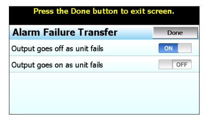
The **Output goes off as unit fails** selection will force the output off during failure regardless of the alarm activation status.
