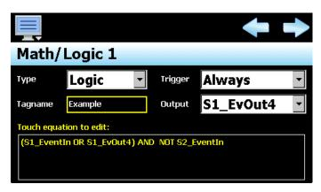
If the loop 1 event input is on and the loop 2 event input is off, the output will be true. Since the output is logically OR'd with the loop 1 event input, even if the input is turned off, the expression within the parenthesis is still true so the output holds itself on.
