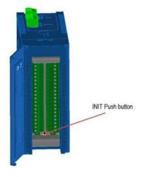
Cycle power to the monitor module after the reset is performed and again press the "Detect Monitor Point Card" button on the MCT4. The MCT4 should then be able to set the proper communication settings. Upon success, be sure to cycle power to the monitor module so that it will begin using the new communication settings.
