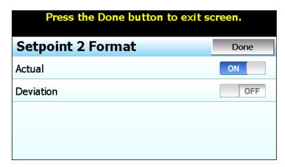
The **Actual** selection means that set point 2 will be an actual set point value, i.e., temperature for example. When the event input is then activated, the value entered for set point 2 (see following section) will be used as the loop set point, overriding the current user entered or operating program set point. When the event input is deactivated, the loop set point will then revert back to the user entered or operating program set point.
