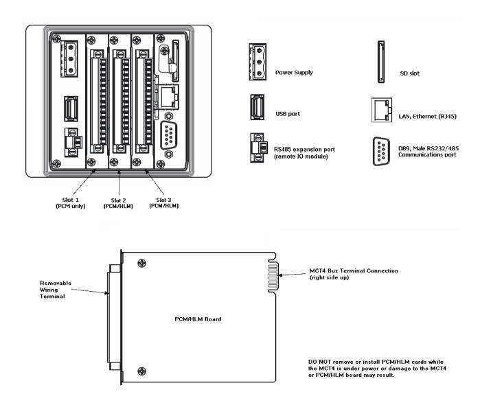
NOTE: The MCT4 will not operate properly without the SD card installed into the SD card slot on the back of the unit. The SD card is preloaded with all software required for 'Auto-Boot' operation. The slot on the back of the interface is 'keyed' so the card can only be installed in one direction. The card is preinstalled for your convenience. If the card is removed, take care when inserting the SD card and DO NOT force it into the slot. The card MUST be installed prior to application of power.
