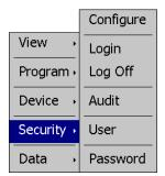
The **Security** menu provides access for user login, security settings and audit trail viewing if the security system is enabled.
