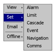
The **Set** menu provides access to settings Alarm set points, control loop set point Limits, Cascade control settings, Event tagnames, Navigation type selection and Communications options.
