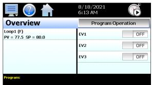
While the timer is not in operation, event 1 can be turned on and off manually by the user. When the timer is running, the event is forced on by the timer. Once the timer completes its cycle, the event will be forced off. To start the timer, simply press the "Stopwatch" icon and the numeric keypad will be displayed. Enter the desired time and press the Start button to begin timer operation (see section 5.1.2.1 Entering the Time and Starting the Timer below).
