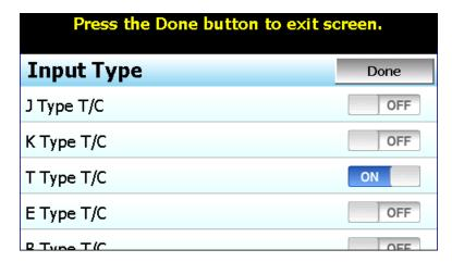
The input type selections are mutually exclusive, i.e., selecting one input will turn all other selections off. Once the desired input type has been selected, press the "Done" button to set the input type for the loop control board and return to the main Loop Configuration screen.
