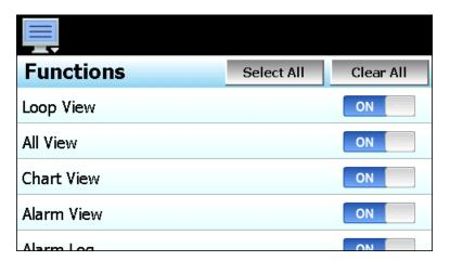
**IMPORTANT:** Disabling MCT4 functions that are not required for the application results in a system that is clean and easy to use for the operator; however, be careful when disabling certain items. Without access to them, there may be no way to determine if the system is operating as required.
