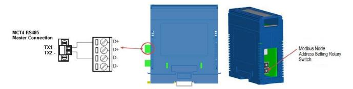
In order for the MCT4 to be able to communicate with the monitor module, the communications address must also be properly set. To do this, remove the cover located on the bottom of the module to access the rotary switches. Adjust both rotatory knobs to a value of 1. Replace the cover after the settings have been made.
