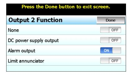
The **DC power supply output** function must be selected when the output type ordered for the limit control is a transmitter power supply.
