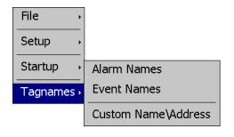
The **Tagnames** menu provides access to the text editing functions of the Configurator which allow the event and alarm names to be changed to match their use in the system. The menu also provides access to edit the splash screen information that is shown when the runtime application starts.
