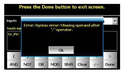
The error message will provide help in determining what is wrong with the equation; however, due to the number of possible combinations it is up to the user to ultimately evaluate the equation and verify its validity. Once the equation can be properly solved, pressing the "Done" button will return to the Math/Logic Configuration screen.
