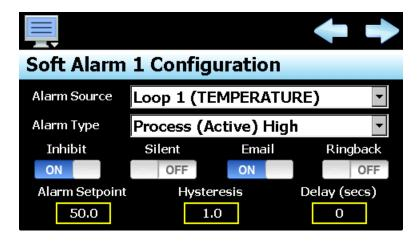
The **Alarm Source** drop down menu selection lists all loops, limits, monitor points and math equations (if configured) to be chosen for the process value to be monitored by the alarm. Any configured logic equations are also included as alarm source selections in which the true/false state of the equation is utilized to activate the alarm.
