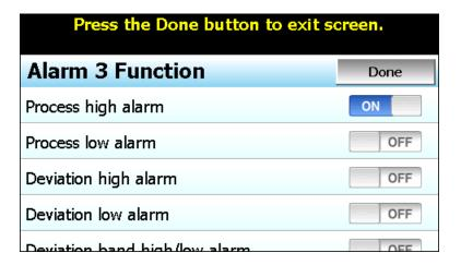
A **Process high alarm** is independent of set point. When the process value is higher than the alarm set point (PV > ASP), a process high alarm occurs. When the process value is lower than the alarm set point minus the alarm hysteresis (PV < ASP–AHY), the alarm is off.
