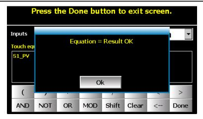
Only a valid equation can be saved. If the equation cannot be properly solved, you will not be able to exit the screen until the equation is corrected or cleared.
