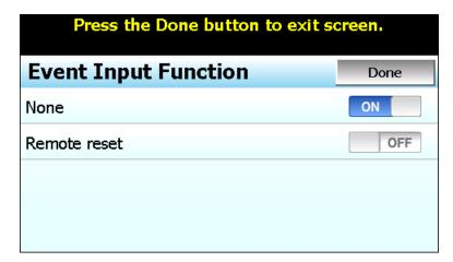
When **Remote reset** is selected for the event input function, the event input will perform an alarm reset each time the input terminals go from open to closed.
