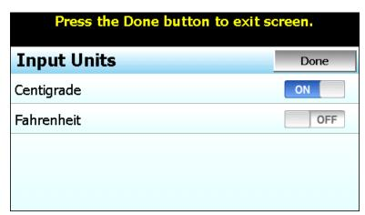
The input unit selections for temperature are mutually exclusive, i.e., selecting one will turn off the other. Once the desired temperature units have been selected, press the "Done" button to set the input units for the limit control and return to the main Limit Configuration screen.
