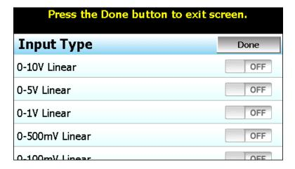
The input type selections are mutually exclusive, i.e., selecting one input will turn all other selections off. Once the desired input type has been selected, press the "Done" button to set the input type for the monitor point and return to the main Monitor Configuration screen.
