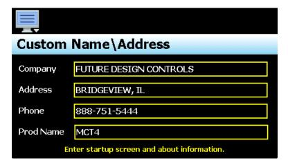
To edit the company, address, phone number or controller (product) name, press the field and enter the desired text. Each field can be entered with a maximum of 24 characters that will be displayed on the splash screen when the MCT4 starts.
