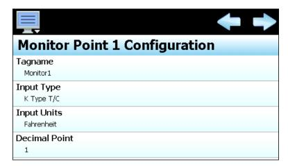
To view all of the available settings for a monitor point, simply swipe up or down on the screen to scroll through the list items. To edit a value, tap the row for the desired item. If the entry is a simple numeric value, the number entry pad will be shown. If the item has multiple selections to choose from, a list of individual selections for the item will be shown.
