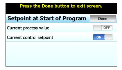
The **Current process value** selection will cause the loop control to immediately assume the current process value as the set point when the program is started. If the program is started on a ramp step, the program will begin ramping the set point from the current process value to the target set point of the step. If the program is started on a soak step, the program will hold the set point at the process value for the duration of the soak step.
