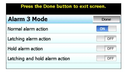
**Normal alarm action** has the alarm output off in the non-alarm condition and on in the alarm condition. The output state is inverted for a reverse alarm output.
