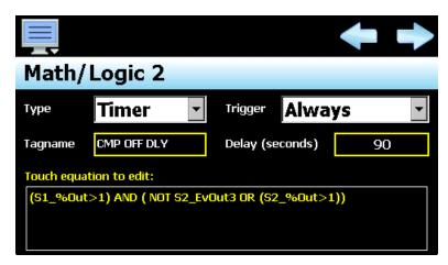
Before utilizing the on and off delay timers in logic equations to active the compressor outputs, one more timer is required. In the case of dual stage refrigeration systems, a delay is required between the start of stage 1 and the start of stage 2. This is necessary in order for the first stage to be ready for the load placed on it when the second stage starts, so that it can remove the heat from the second stage. Thus, we require one more timer which will create in math/logic equation 3.
