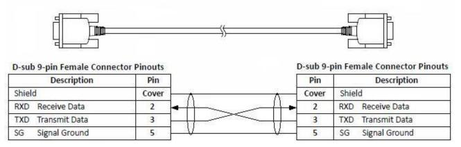
**NOTE:** DO NOT use a standard null-modem cable to connect the MCT4 to a PC. Most computers do not provide a standard serial port and a USB to serial converter must be used. Incompatibilities may exist between the MCT4 and certain USB to serial adapters which may cause the MCT4 to malfunction when connected using a standard null-modem cable.
