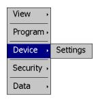
The **Device** menu provides access to the MCT4 controller settings. These include, loop set point entry limits, alarm set points, communication settings, email setup as well as access to offline settings for date/time, etc.
