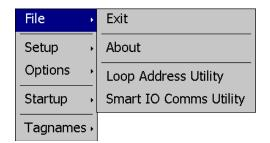
The **File** menu provides selections of "Exit" and "About". The exit function for the Configurator saves all settings and closes the Configurator application. The about selection displays version information for the Configurator application and configured control devices.
