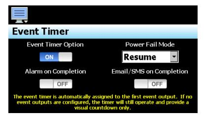
The Event Timer Option button toggles the option on and off. When enabled, the timer is automatically associated with event 1 and its corresponding output. Thus, when the timer is started, event 1 will be turned on. When the timer is stopped and/or completes its cycle, event 1 will be turned off. Access to the timer is provided by a "Stopwatch" icon on the Loop View and Overview screens in the runtime application.
