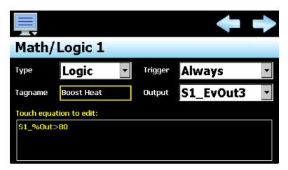
When the temperature percentage of output is greater than 80, event output 3 of loop 1 will activate. When the percentage of output is below 80, the output will turn off. The equation for boost cool will be entered in the same manner. First, press the "next" navigation arrow at the top right of the screen to access equation 2.
