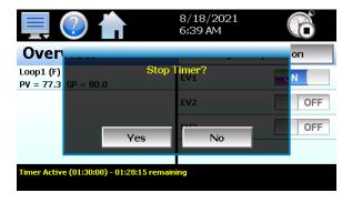
**NOTE:** Timer operation and automatic program operation cannot be performed at the same time. If the timer is active, an automatic ramp/soak program cannot be started. Likewise, if an automatic ramp/soak program is in operation, the timer cannot be activated.
