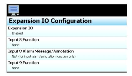
To view all of the available settings, the Expansion IO must be set to "Enabled". When enabled, the configuration items for each input and output will then be provided in the list. Simply swipe up or down on the screen to scroll through the list items. To edit a value, tap the row for the desired item.
