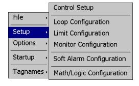
The **Setup** menu provides access to the control setup options. These options include the controller type (single loop, dual loop, cascade, etc.), the process loop and limit settings, soft alarm settings, monitor point settings and math/logic equation entry.
