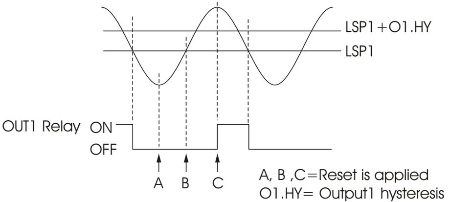
Figure 1-5 Low Limit Operation
