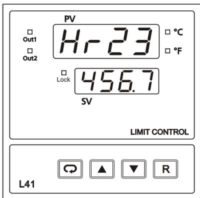
Display the hours used for 1.5 seconds. The left diagram shows that the unit has been used for 23456.7 hours since production.
