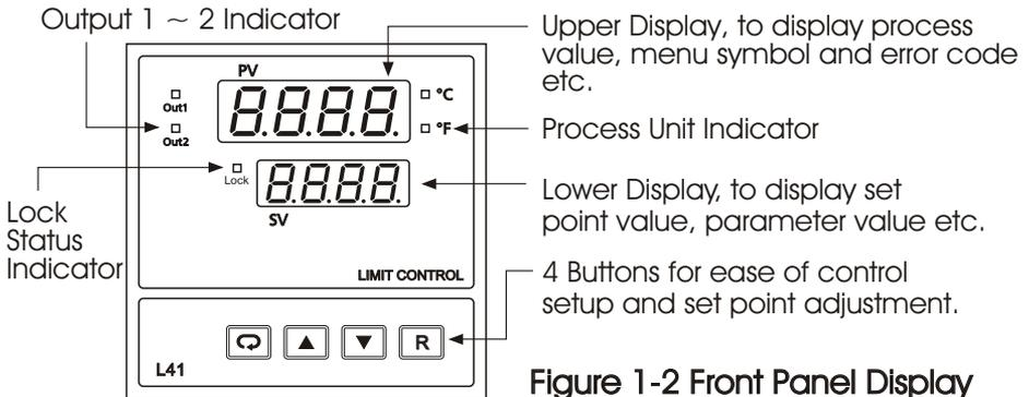
Figure 1-2 Front Panel Display
