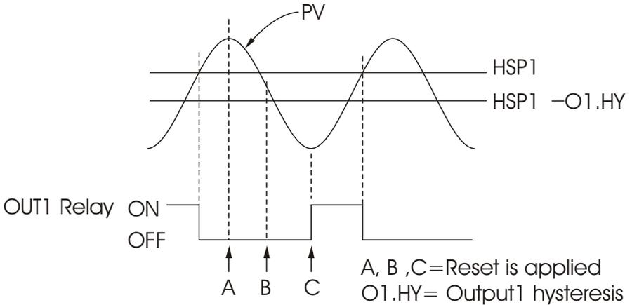
Figure 1-4 High Limit Operation
