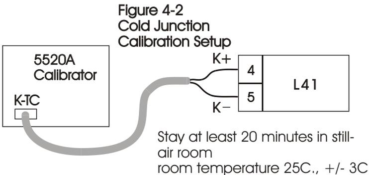
The 5520A calibrator is configured as K, Celsius type thermocouple output with internal compensation. **Send a 0.00 C signal to the unit under calibration.**
