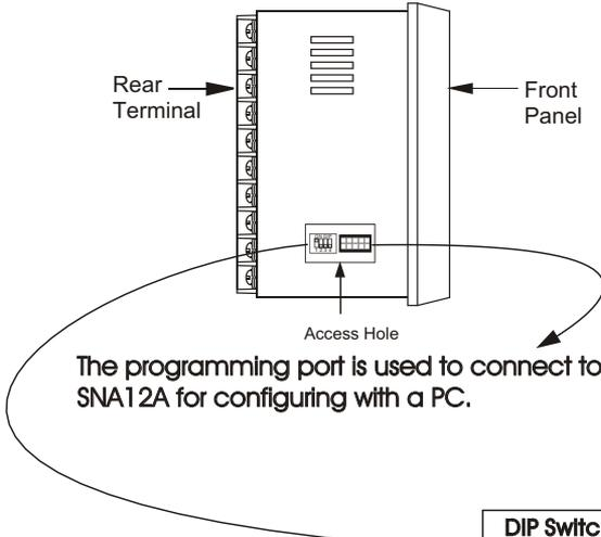
The programming port is used to connect to SNA12A for configuring with a PC.
