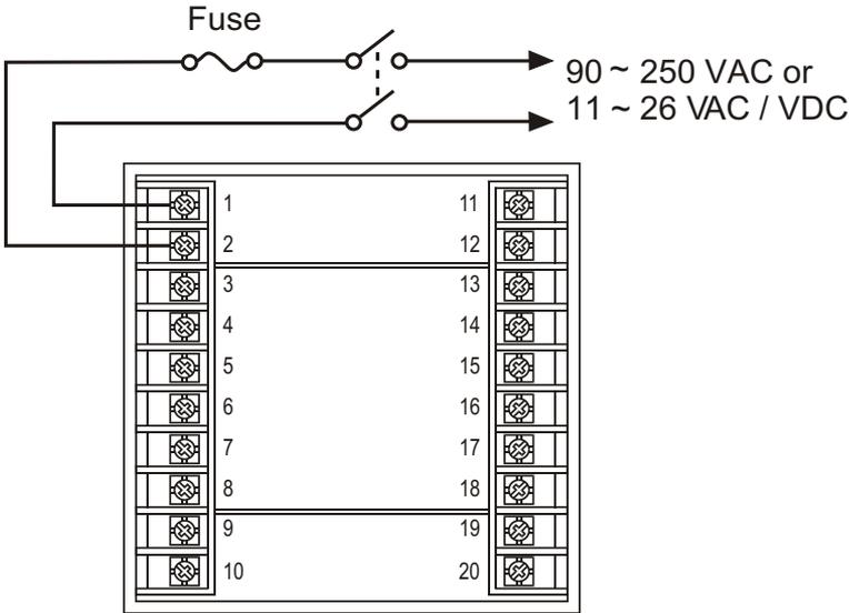
Figure 2-4 Power Supply Connections
