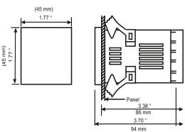
Figure 6.1 Mounting Dimensions
