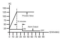
The dwell function may be used to operate an external device such as a siren to alert when a soak time has been reached.
