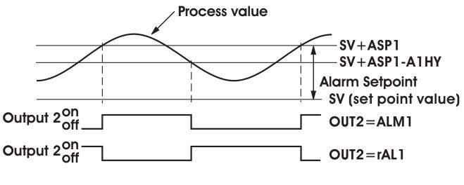
Figure 3.6 Deviation High Alarm 1 Operation
