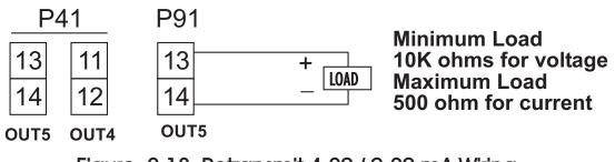
Figure 2.18 Retransmit 4-20 / 0-20 mA Wiring
