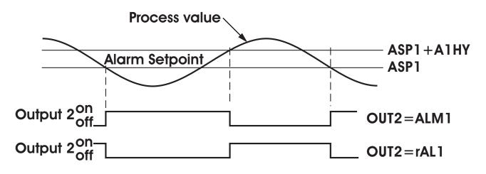
Figure 3.5 Process Low Alarm 1 Operation
