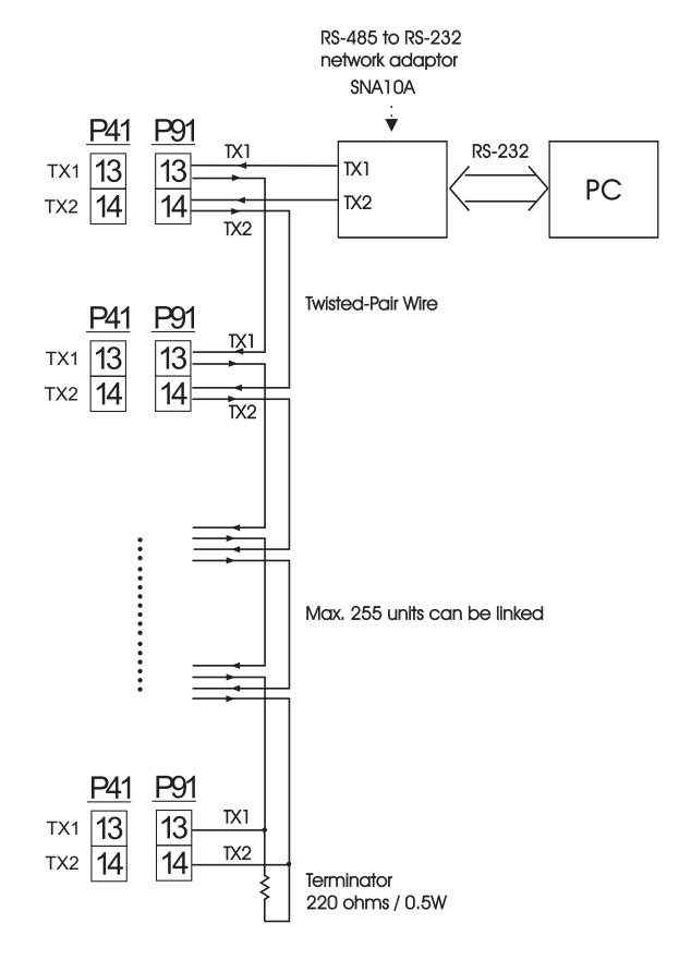
Figure 2.19 RS-485 Wiring
