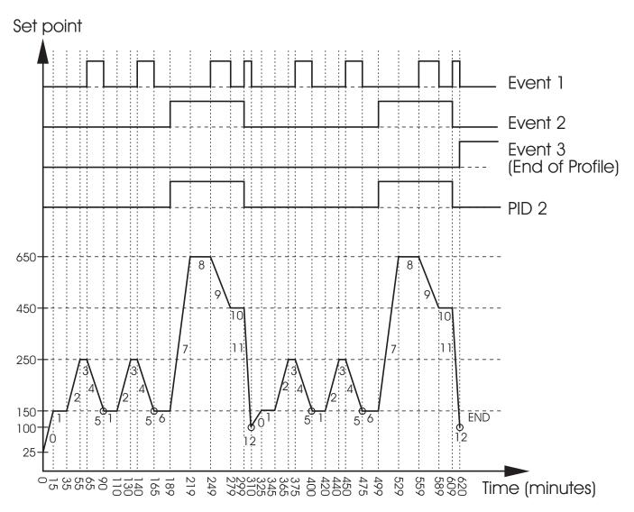
A heat treatment oven needs to vary temperature as a function of time according to the process graph depicted above. Output 1 of the control is used as the heating output, but due to the high rate of heating required, an additional heater is turned on at elevated temperatures using event 1 (output 2) to act as a boost. When the boost heater is activated, a second PID set is also required in order to maintain proper temperature control of the oven.
