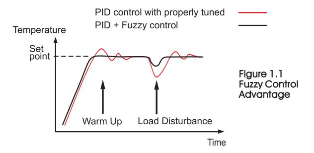
The "P" series can be configured as a single set point controller (static mode) or a ramp and dwell profiling controller (profile mode). The profile mode feature allows the user to program up to 9 profiles of up to 64 free-format (ramp, dwell, jump or end) segments each. The total segments available for the product is 288 segments. NOTE: Profiles can NOT be linked together.
