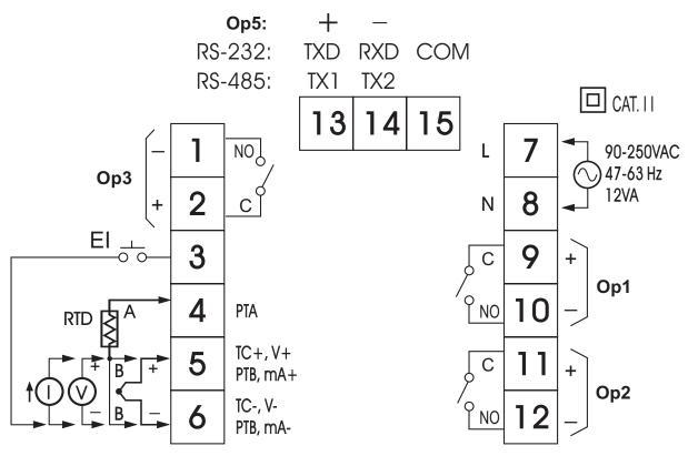
50C max. air ambient Use copper conductors (except on T/C input )
