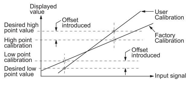
Figure 3.9 Two Point User Calibration
