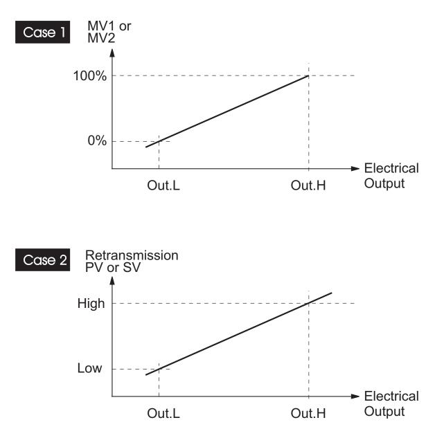
Figure 3.12 Output Scaling Function
