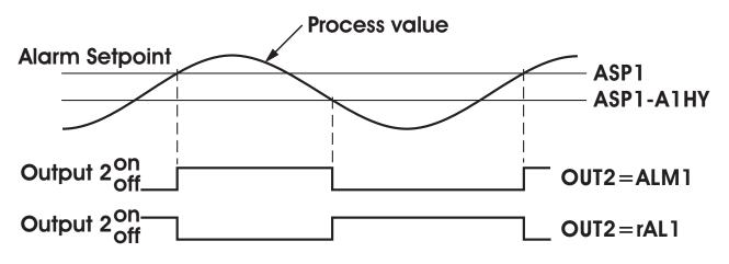
Figure 3.4 Process High Alarm 1 Operation
