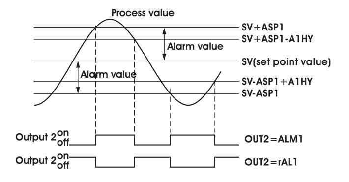
Figure 3.8 Deviation Band Alarm 1 Operation
