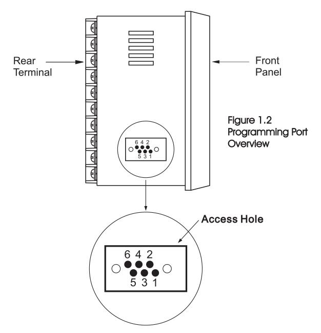
A special connector (CC91-1) is used to connect the programming port to a PC for automatic configuration. The PC must have FDC-Set installed to use the configuration feature via PC.
