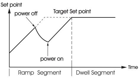
Figure 4.6 Recovery from PV at Ramp Segment
