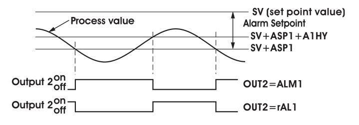
Figure 3.7 Deviation Low Alarm 1 Operation
