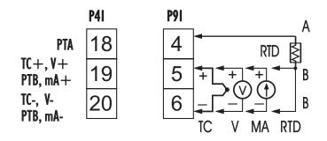
Figure 2.7 Sensor Input Wiring
