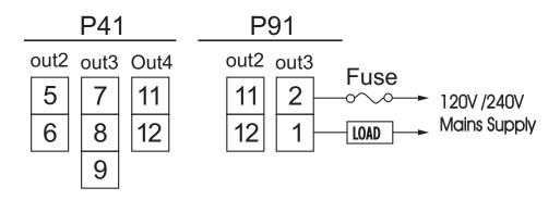
Figure 2.16 Alarm/Event Output Wiring
