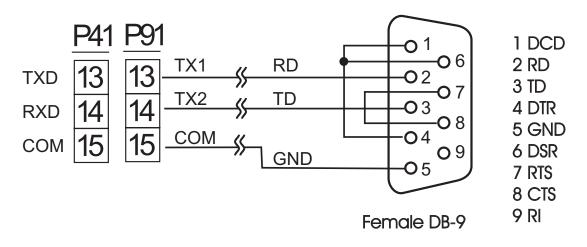
Figure 2.21 Configuration of RS-232 Cable
