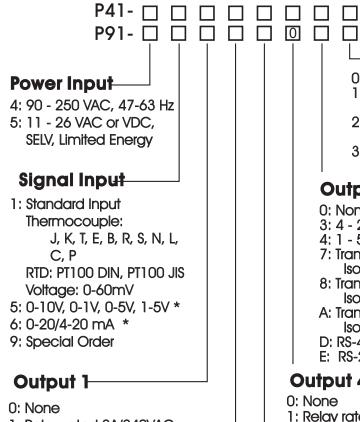
1: Relay rated 2A/240VAC 2: SSR Driver 5 VDC @ 30 Ma 3: 4 - 20mA / 0 - 20mA Isolated 4: 1 - 5V / 0 - 5V/0 - 10V Isolated 6: Triac output 1A / 240VAC,SSR C: SSR Driver 14 VDC @ 40 Ma 9: Special order
