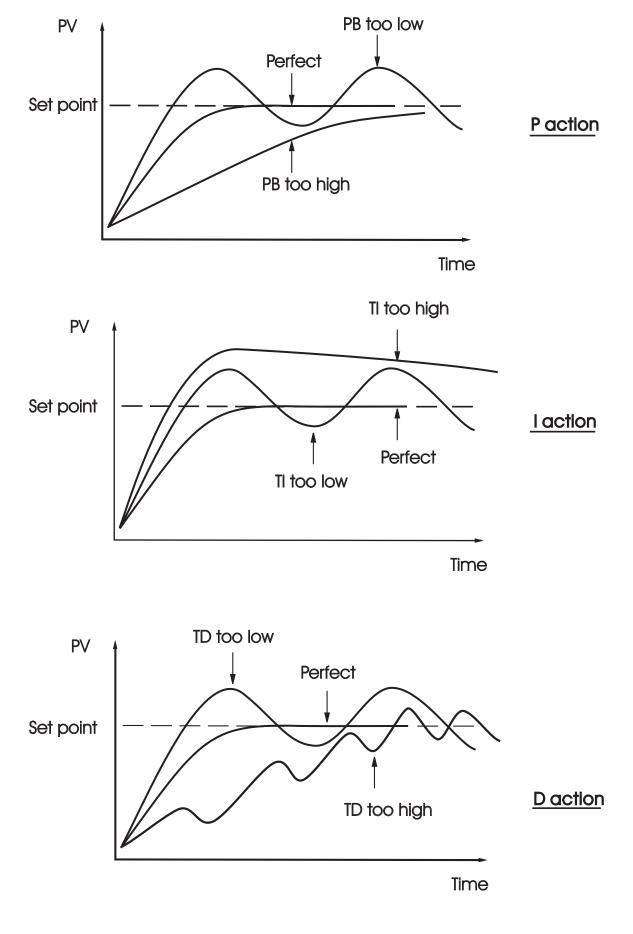
Figure 3.11 Effects of PID Adjustment
