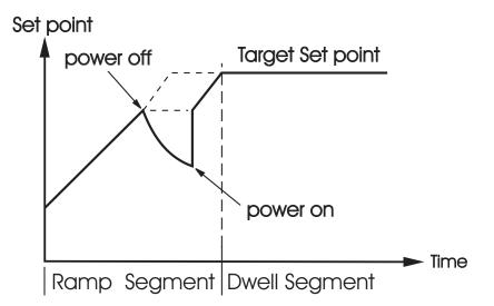
Figure 4.4 Recovery from Profile at Ramp Segment
